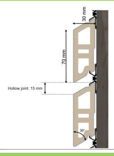
Weight of a profile: 1.80 kg per metre run
