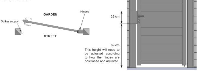
The screws supplied fix the striker to the striker support, and the support to the aluminium post. The inserts are to be riveted to the aluminium posts, after pre-drilling Ø8 mm holes. If installing on a masonry pillar, use Ø4 mm screws with suitable screw anchors.
